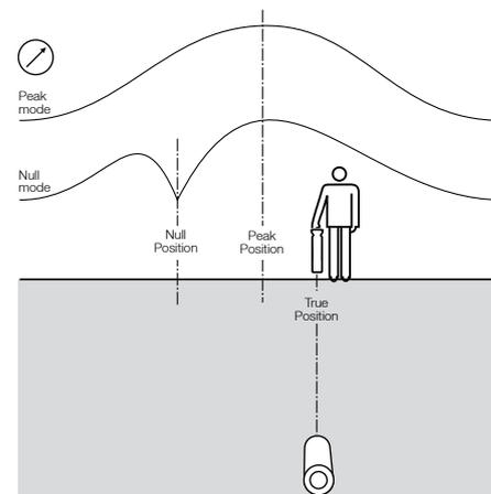
1. With the antenna perpendicular to the line, make traverses across the line. Define the point of maximum response.
