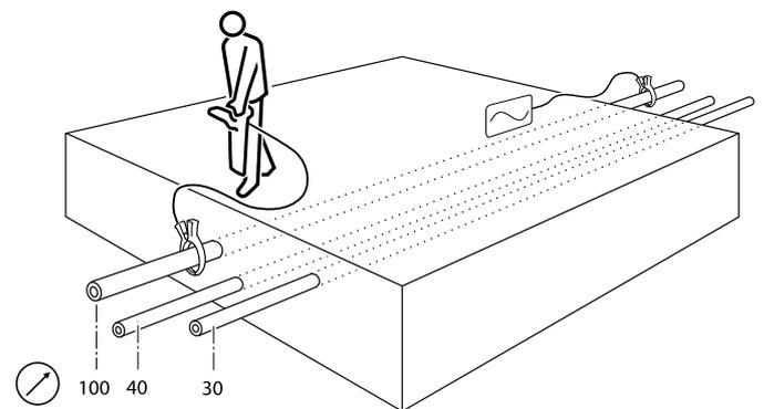
To ensure that the target cable has been correctly identified, reverse the positions of the transmitter and locator and check that the strongest response is still received from the target cable by the locator in its new position.
