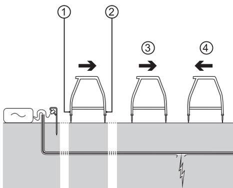
If you are trying to locate high resistance faults or there is a long distance between faults, carry on with the survey and the locator will lock on when you get closer to the fault.
