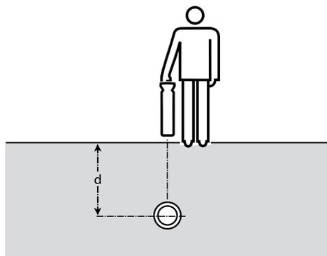
To avoid signal distortion, do not apply the signal by induction. If direct connection or signal clamping is not possible, place the transmitter at least 15m (49ft) from the point of any depth measurements.
