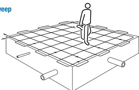
Stop when the locator response rises to indicate the presence of a line. Pinpoint the line and mark its position. Trace the line out of the area being searched. Resume grid search in the area.
