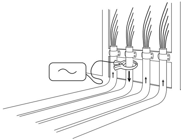
**NOTE:** It is not necessary to make a ground connection from the transmitter when using the clamp.
