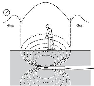
Figure 10.8: Calculating sonde depth
