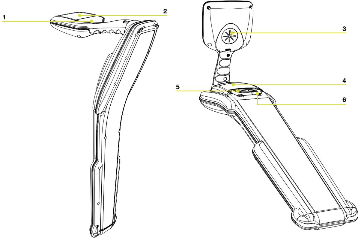
Figure 2.2: RD8000 showing Bluetooth® antenna
