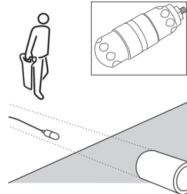
Insert the Mouse approximately 1m/3yd into the duct or drain and adjust the C.A.T<sup>3</sup> sensitivity to receive the signal.
