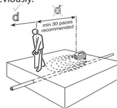
Hold the C.A.T<sup>3</sup> still, vertical and at right angles to the buried line. Momentarily depress the depth button. The display will show a moving clockface followed by the depth measurement.
