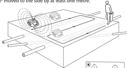
Alternatively, use a two man technique to search an area for buried utilities as shown.
