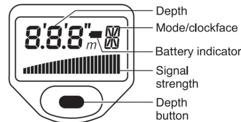
The main features of the C.A.T<sup>3</sup>V and C.A.T<sup>3</sup>+ are the same as the C.A.T<sup>3</sup> but the addition of a liquid crystal display brings further features.
