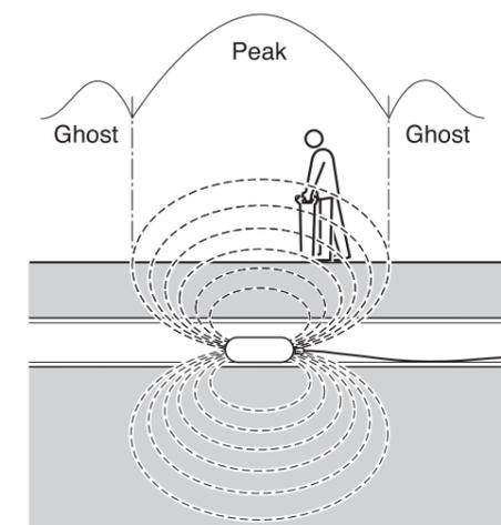
Rotating the C.A.T<sup>3</sup> about it's axis to obtain the largest signal puts the blade of the C.A.T<sup>3</sup> in line with the Mouse and is a good way of identifying the direction of the duct or pipe.
