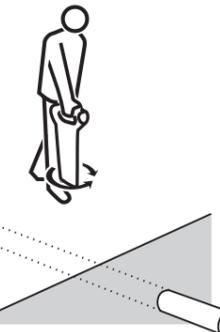
The presence of a buried metallic pipe or cable will be indicated by a tone emitted from the speaker. Keep the blade of the C.A.T<sup>3</sup> vertical and move slowly backwards and forwards over the cable or pipe, reducing the sensitivity for a narrower response. If using a C.A.T<sup>3</sup>V or C.A.T<sup>3</sup>+ use the meter deflection to aid pinpointing. Maximum meter deflection indicates the position of the conductor.
