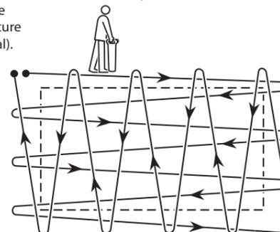
Trace the buried conductor keeping the C.A.T<sup>3</sup> vertical and moving it steadily from side to side. Follow the line of the buried conductor marking it with chalk or paint across the area to be excavated.
