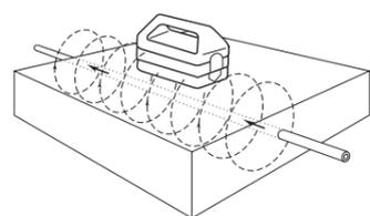
Start tracing the target line at least five paces from the Genny<sup>3</sup> with the C.A.T<sup>3</sup> set in the Genny mode. Working too close to the Genny<sup>3</sup> may give false readings as the C.A.T<sup>3</sup> will detect radiated signals directly from the Genny<sup>3</sup> rather than the target line.
