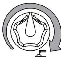
The welding current is regulated by turning knob "T" continuously. If set to the minimum (turned fully in an anticlockwise direction) it provides a current of approximately 30 A; if set to the maximum (turned fully in a clockwise direction) it gives a maximum current of approximately 600A.
