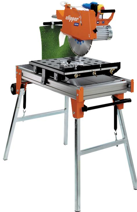
The **Clipper CHW Modulo** is a lightweight, modular masonry saw designed for the on-site cutting of bricks, tiles, paving slabs and similar building materials. The CHW is made from interchangeable extruded aluminium profiles, resulting in a high strength/performance machine at low weight. The CHW features a 2.2kw direct drive motor, which can be run via a 3 KVA transformer or 13 amp domestic supply.
