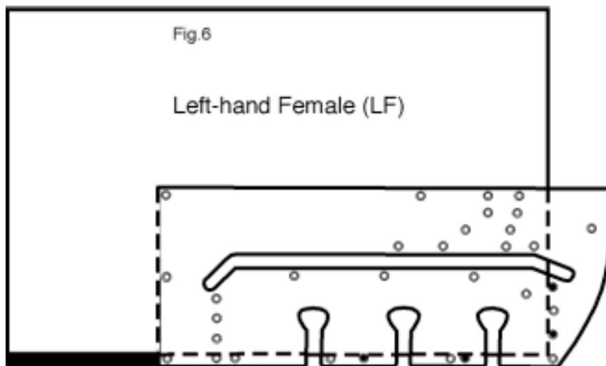
Offer the jig up to the *worktop* and clamp into position. Set your plunging depth to about 20mm. You should ensure this is sufficient to accommodate your joining bolt. Now use each mushroom shaped recess to guide the router. Working clockwise around the slot, remove all the waste. *Note*; worktop widths 400-550mm will only accommodate 2 slots.
