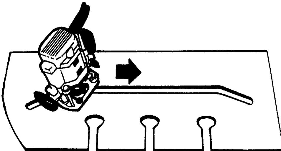
***It is important that you work the router from left to right. To work the router right to left means working against the cutter's direction, which will cause the router to travel away from you and may damage the jig or even cause injury.***
