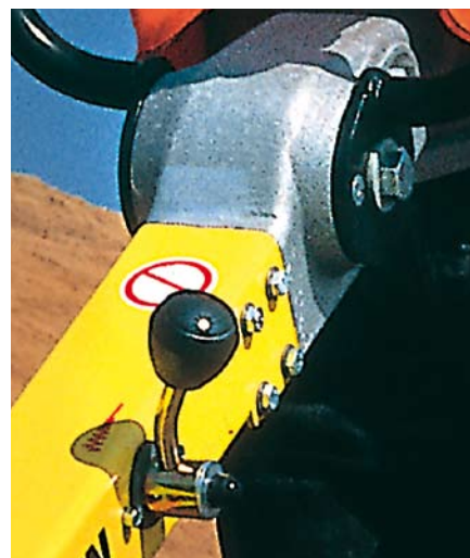
Throttle control at operator's handle
