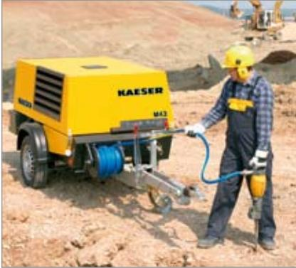
MOBILAIR portable compressor models with free air deliveries ranging from 2 to 5.6 m<sup>3</sup>/min ensure dependable performance even in cold conditions: KAESER's patented Anti-Frost Control automatically adjusts operating temperature according to ambient temperature. This system is therefore particularly useful at times of the year when ambient temperatures are lower, as it protects air tools against freezing and significantly enhances both system availability and service life.
