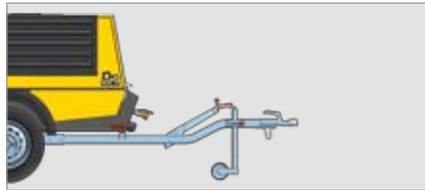
Fixed towing hitch without run-on brake and with parking brake
