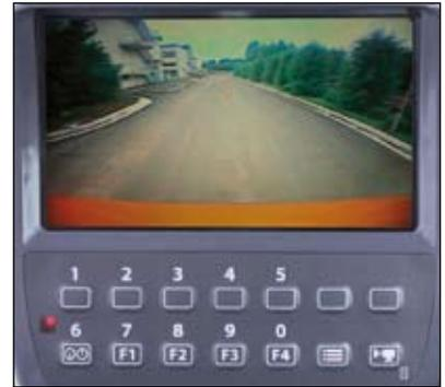
The widescreen color LCD, teamed up with the rear view camera on the counterweight, gives the operator unobstructed rearward viewing. The rear view camera automatically works when traveling, and can also be manually turned on with a select switch on the monitor.
