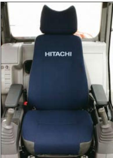
Wide adjustable armrests and a retractable seat belt are included. Short stroke levers allow for continuous operation with less fatigue. Three switches on the lever (optional) can be set to operate attachments other than buckets. The cab is pressurized to keep out dust. Noise and vibrations are kept to a minimum due to the elastic mounts, filled with silicone oil, the cab rests on.
