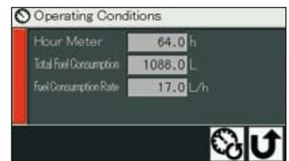
Fuel consumption per operating hour is computed, and the result is displayed on the LCD monitor. This information suggests refuelling timing, and guides energy-saving operation and efficient job management.
