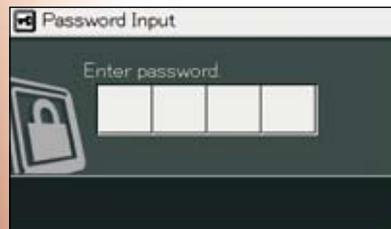
The electronic immobiliser requires the entry of an encryption code to the multifunctional monitor each time when starting the engine to prevent theft and vandalism.
