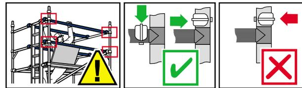
Ensure horizontal braces and guardrails are fitted correctly. Always fit as shown.
