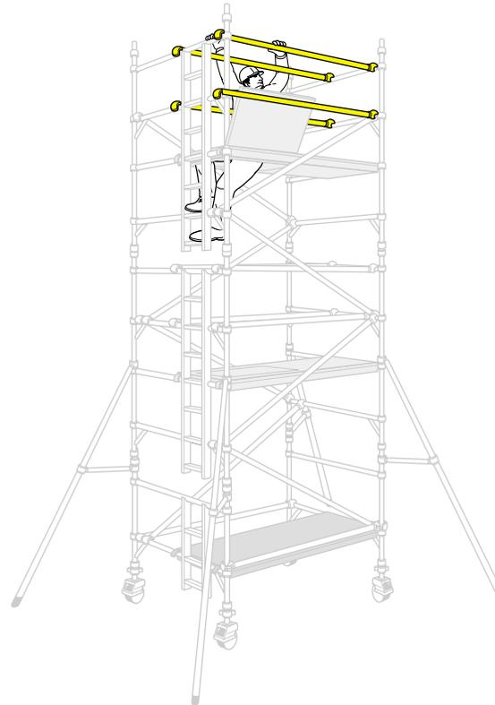
Continue until the required height is reached. Reposition the fixed deck to the required platform height and fit a trapdoor deck alongside it as shown in **stage 7**. Fit a single diagonal at the top of the tower as shown in **stage 7**. Fit the final guardrails as shown in **stage 7**.
